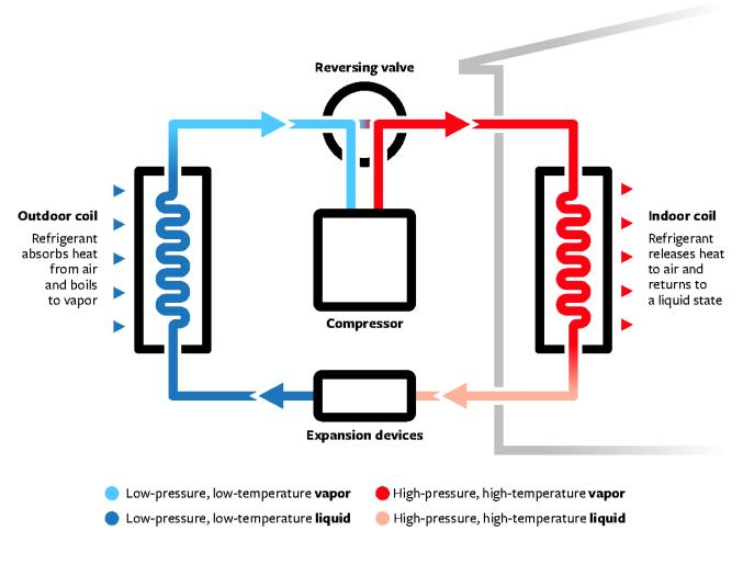
Figure 3: How heat pumps operate
