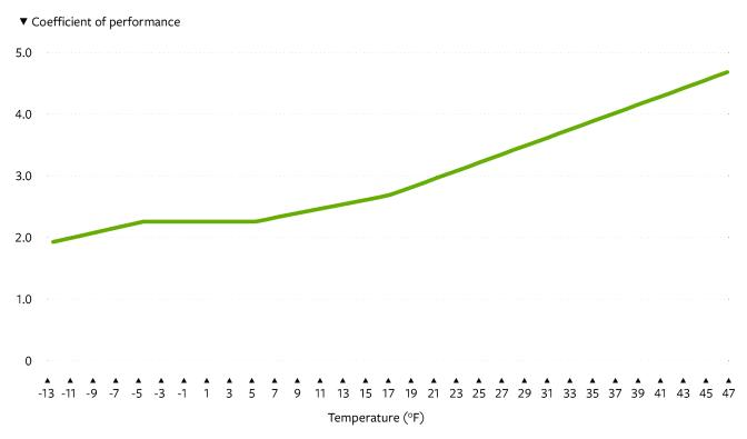
Figure 4: Impressive performance of a leading air-source heat pump, with performance determined by temperature. Source: Mitsubishi product specification sheet.
